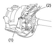
(1) brake lever adjusting nut
