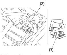
(2) fuse holder assembly(3) fuse holder
