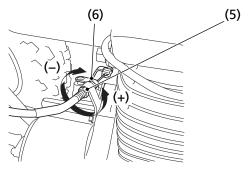
(5) lower adjusting nut(6) lower lock nut
