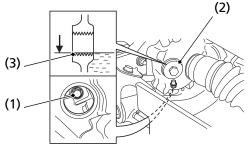
(1) oil drain bolt (2) oil fill cap (3) oil fill inspection hole
