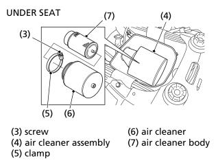
11. Install the air cleaner on the air cleaner body.
