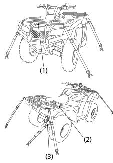
(1) front cargo rack (2) rear cargo rack (3) trailer hitch
