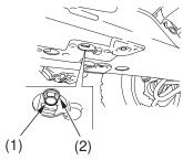
(1) engine oil drain bolt
