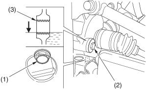
(1) oil drain bolt(2) oil fill cap
