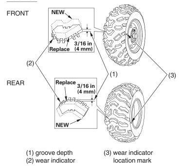
To check the condition of a tire tread, measure the groove depth (1) in the center of the tire, or check the wear indicator (2).
