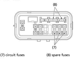
6. To check or replace a circuit fuse (7), pull the old fuse out of its retaining clips with fuse puller on the underside of the rear fender cover (page 113).
