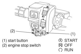
The start button (1) is used for starting the engine. Pushing the button in starts the engine. See *Starting Procedure*, page 61.
