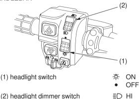
The headlight switch (1) is used to turn the headlight ON (♣) or OFF ( • ). To operate, turn the switch to ON (♣) or OFF ( • ).
