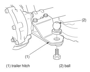
The trailer hitch (1) is located on the rear axle housing. To use the hitch, you'll need a proper size ball (2) as specified by the trailer manufacturer.
