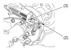
(2) brake lever adjusting nut
