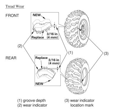
To check the condition of a tire tread, measure the groove depth (1) in the center of the tire, or check the wear indicator (2).
