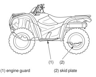
The engine guard (1) protects the frame and engine crankcase. The skid plate (2) protects the rear final gear case. Check the guard and plate for cracks, damage or looseness at intervals shown in the Maintenance Schedule.
