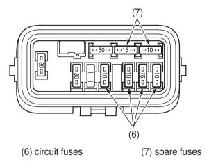
6. To check or replace a circuit fuse (6), pull the old fuse out of its retaining clips.
