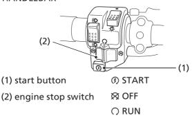
The start button (1) is used for starting the engine. Pushing the button in starts the engine. See *Starting Procedure*, page 73.
