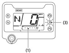
(1) coolant temperature gauge (3) high coolant temperature indicator
