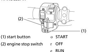
The start button (1) is used for starting the engine. Pushing the button in starts the engine. See *Starting Procedure*, page 74.
