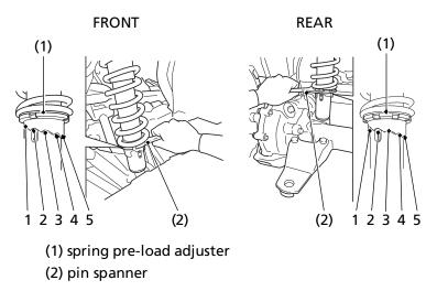
The spring pre-load adjuster (1) has 5 positions for different load or riding conditions.
