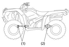
(1) propeller shaft boots (Except TRX420TM1)(2) yoke joint boot
