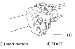
The start button (1) is used for starting the engine. Pushing the button in starts the engine. See *Starting Procedure*, page 47.
