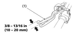
(1) clutch lever/parking brake lever
