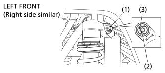
(1) compression damping adjuster(3) reference punch mark(2) punch mark
