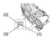
(1) rebound damping adjuster(3) reference punch mark(2) punch mark
