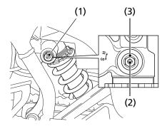
(1) compression damping adjuster (3) reference punch mark
