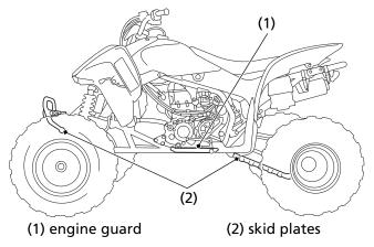
The engine guard (1) protects the engine crankcase. The skid plates (2) protect the frame/lower arm, the drive components and the rear brake. Check the guard and plates for cracks, damage or looseness at intervals shown in the Maintenance Schedule.
