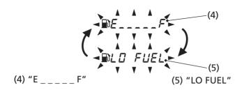
When the fuel gauge show "E  $\_$  F" (4) and "LO FUEL" (5) blink 3 times alternately and fuel mark blinks, you should refuel as soon as possible.
