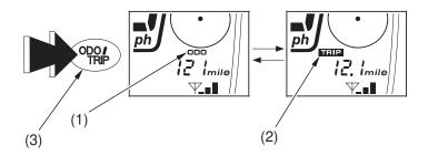
To reset the tripmeter to zero, press and hold the odometer/tripmeter select button for more than 2 seconds.
