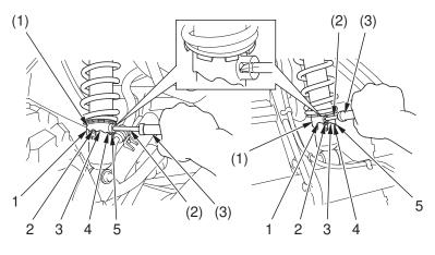
(1) spring pre-load adjuster(3) screwdriver handle(2) standard/Phillips screwdriver
