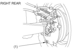
(1) rear brake drain bolt
