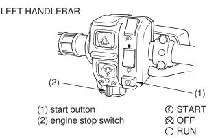
The start button (1) is used for starting the engine. Pushing the button in starts the engine. See *Starting Procedure*, page 71.
