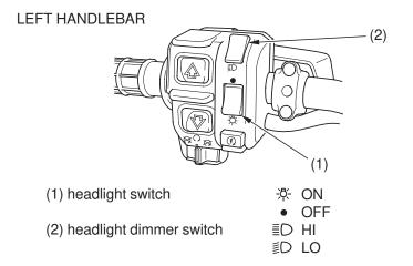
The headlight switch (1) is used to turn the headlights and assist headlight ON ( $\Rightarrow$ ) or OFF ( $\bullet$ ). To operate, turn the switch to ON ( $\Rightarrow$ ) or OFF ( $\bullet$ ).
