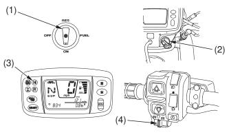
(1) fuel valve(2) ignition switch(3) neutral indicator(4) engine stop switch
