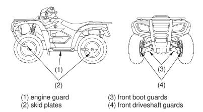
The engine guard (1) protects the engine crankcase, and the skid plates (2) protect the frame and rear final gear case.
