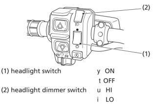
The headlight switch (1) is used to turn the headlights and assist headlight ON (y ) or OFF (t). To operate, turn the switch to ON (y ) or OFF (t).
