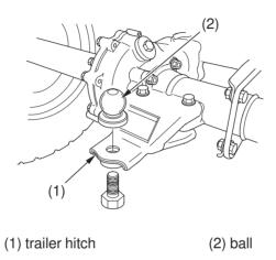
The trailer hitch (1) is located on the rear axle housing. To use the hitch, you'll need a proper size ball (2) as specified by the trailer manufacturer.
