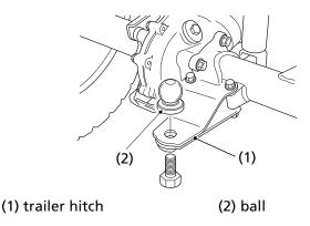
The trailer hitch (1) is located on the rear axle housing. To use the hitch, you'll need a proper size ball (2) as specified by the trailer manufacturer.
