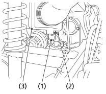
(1) drain tube(3) air cleaner housing(2) clip
