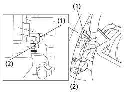
Check the wear indicator (1). If the wear indicator aligns with the edge of the reference mark (2), both pads must be replaced, see your dealer for this replacement.
