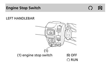
The engine stop switch (1) is used to stop the engine in an emergency. To operate, slide the switch to the OFF  $(\mbox{\ensuremath{\bowtie}})$  position. The switch must be in the RUN  $(\mbox{\ensuremath{\cap}})$  position to start the engine, and it should normally remain in the RUN  $(\mbox{\ensuremath{\cap}})$  position even when the engine is OFF.
