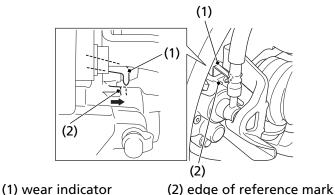
Check the wear indicator (1). If the wear indicator aligns with the edge of the reference mark (2), both pads must be replaced, see your dealer for this replacement.
