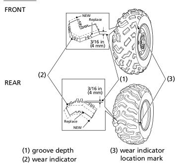
To check the condition of a tire tread, measure the groove depth (1) in the center of the tire, or check the wear indicator (2). For best performance, you should replace a tire before the tread depth at the center reaches the following limits:
