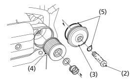
(2) oil filter bolt(3) oil filter cover
