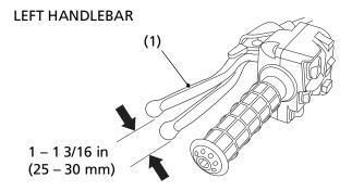
(1) rear brake lever/parking brake lever
