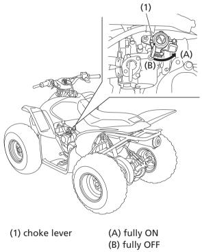
The choke lever (1) may be used when starting the engine. See page 56.
