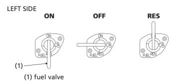
The manual fuel valve (1) is located on the left side under the fuel tank.
