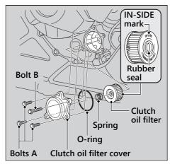
**3.** Install a new clutch oil filter with the rubber seal facing in, toward the engine. You will see "IN-SIDE" mark on the clutch oil filter body, near the seal.
