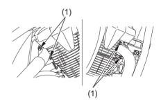
(1) exhaust pipe joint nuts
